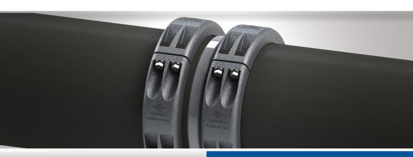
PT's **HD2 LAY FLAT HOSE FITTINGS** offers a quick and economical way to use lay flat hose in the transfer of fluid, typically in fracking operations. The lay flat hose is connected to the HD2 bodies by use of segmented bolt clamps or grooved crimp sleeves. Additional applications include municipal water pumping/bypass and fluid transfer operations.
